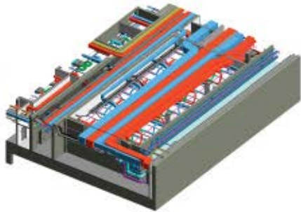
LOD 300 Modeling Secondary Connections of MEP Elements
